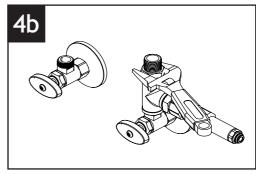
Install brass tee, pressure limiting and dual check valve onto the cold-water supply stop valve. Apply Teflon tape or thread sealant to all threaded joints. Do not overtighten.
