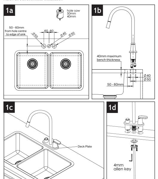
Maximum bench thickness is 40mm. Drill two 50mm diameter holes and one 40mm hole as shown in Step 1a.
