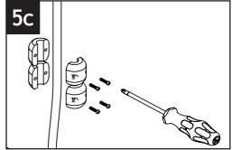
Weights shall be installed approx 450mm below the bench and free of obstruction. Tighten the screws and check to make sure they don't slip. Test the pullout function by pulling the hand piece down while swiveling the spout from left to right, adjust the height of the weights if necessary.
