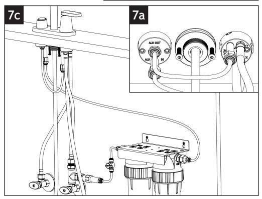
Connect the filter unit outlet to the "ALK in" port under the On/Off button. Trim off any excess tubing and keep all the connections under the sink neat and tidy.
