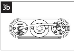
Use a tube cutter, cut approximately 300mm of the 1/4" tubing. Connect the "ALK OUT" port from the left-hand side of the tap to the "ALK" port on the right-hand side.
