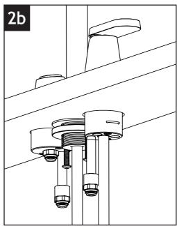
Insert the loose end of the pullout hose into the center port of the mixer body, carefully push the hose all the way in then lock it with the slide pin. Pull the hose down gently to check if it's locked in place. If there is too much resistance for the hose to go in, grease the o-ring seal inside the mixer body.
