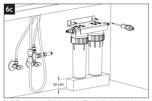
Raise the filter unit using a piece of timber that's thicker than 50mm, place it in a desired location that meets the minimum clearance requirement. Mark and drill the screw locations, then fasten the unit with the mounting screws supplied.
