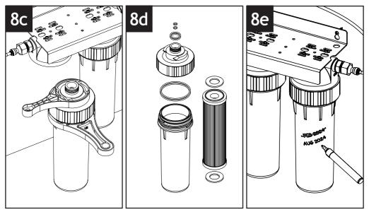
Lock the smaller housing cap wrench onto the top of the housing, then turn the housing wrench to unscrew the top cap from the housing. Replace the cartridges, check, replace and lubricate all the o-rings and seals if necessary. Reinstall the housings by reversing the steps above. Turn cold water back on and mixer tap to full cold, vent and flush the system. Record the date of cartridge replacement on the housing with a permanent marker.
