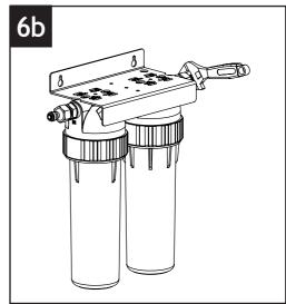
Install the brass hex nipple and 1/4" tube fittings onto both the inlet and outlet of the filter unit. Apply Teflon tape on all the threads, do not overtighten the fittings.
