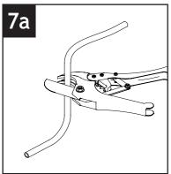
Estimate then cut a length of tubing to connect the outlet of the pressure limiting and dual check valve to the filter unit's inlet. Then cut that tubing in half and install an isolation ball valve in between.
