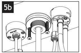
Connect the hot & cold braided supply hoses from the stop valves to their corresponding ports on the mixer body marked "H" and "C".
